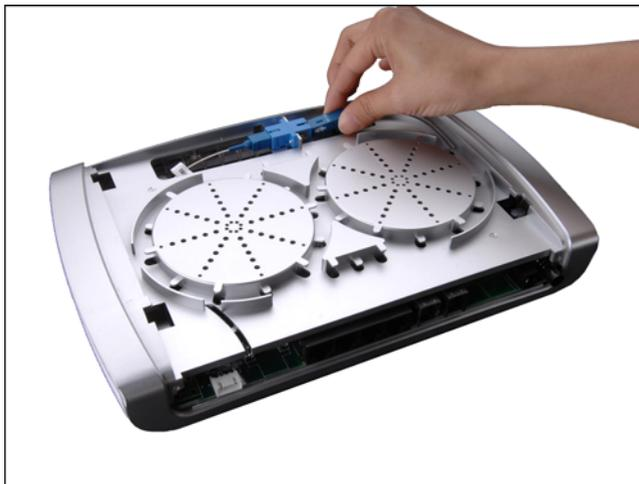
**Step 4** Wind the fiber around the fiber spool.
