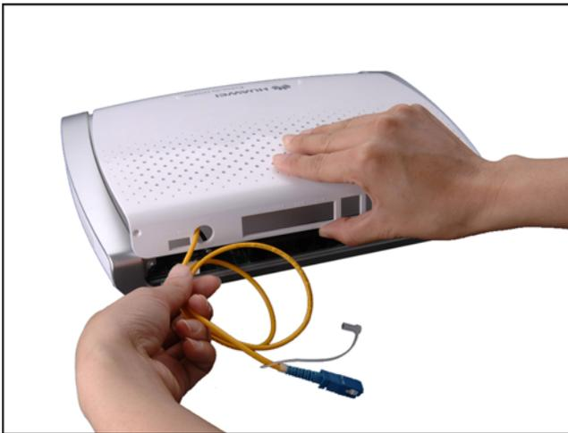
**Step 6** Fix the cover properly and install the rubber plug.
